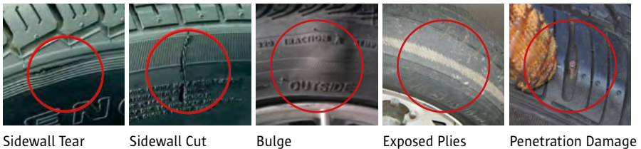
Figure 6: Examples of Tyre Damage/Wear
