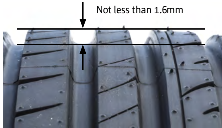
Figure 3: Tyre tread depth
